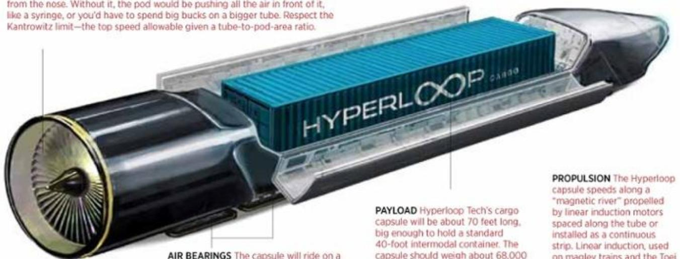
**AIR BEARINGS** The capsule will ride on a cushion of air pumped from the bottom of lunch-tray-size sleds. Landing gear may need to be deployed as it comes to a stop.
